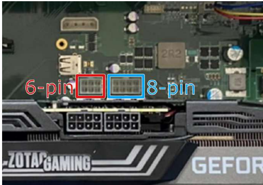
6/ 8-pin power connector on daughter board
