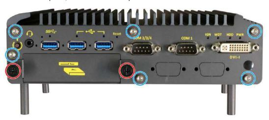
4. Remove the screw indicated on the rear I/O panel and separate it from the enclosure.
