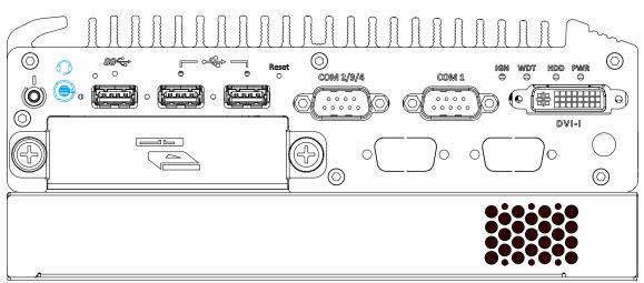
There is a female 4-pole <sup>O</sup>audio jack for headphone (speaker) output and microphone input. To utilize the audio function in Windows, you need to install corresponding drivers. Please refer to the section, <u>Driver Installation</u>.
