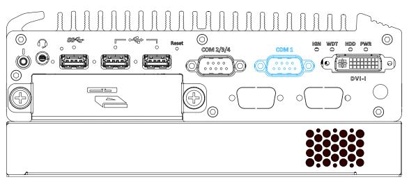
Isolated with up to 15kV ESD protection, the port is implemented using industrial-grade ITE8786 Super IO chip (-40 to 85°C) and provides up to 921600 bps baud rate.COM1 is aRS-485 port via 9-pin D-Sub male connector. The following table describes the pin definition of COM ports.
