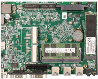
5. Gently press down and secure the module with an M3 P-head screw.
