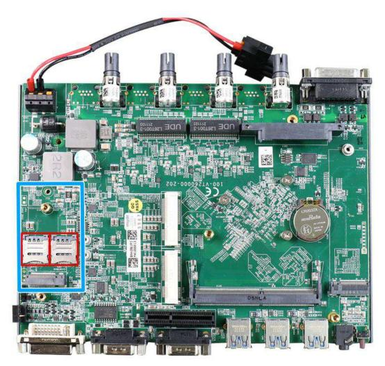
The system has one M.2 3042/ 3052 B key socket (in **blue**) for 5G/4G module installation and dual SIM slots (in **red**). The M.2 slot features USB3.1 and USB 2.0 signal.
