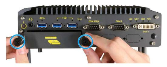
Gently pull out the 2.5" HDD/SSD tray. With HDD/SSD label downwards, secure the HDD/ SSD using the screws provided (indicated in blue), there are two screws on each side.
