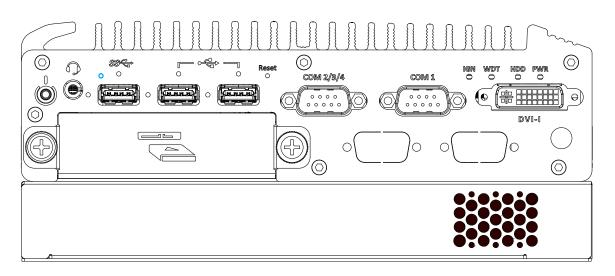
The CMOS Reset button is used to manually reset the motherboard BIOS in case of system halt or malfunction. To avoid unexpected operation, it is purposely placed behind the panel. To reset, please use the tip of a pen, press and hold for at least 5 seconds to reset the BIOS.
