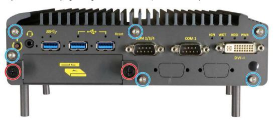
6. Secure the screws (indicated in **blue**) on the M12 connector panel.
