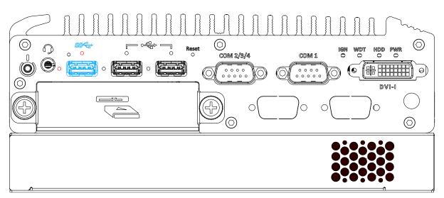
The system offers one USB3.1 Gen1 (SuperSpeed USB) port on its front panel with screw-lock mechanism (indicated in **red**). It is backward-compatible with USB 2.0, USB 1.1 and USB 1.0 devices. Legacy USB support is also provided so you can use USB keyboard/mouse in DOS environment while USB 3.1 Gen1 driver is supported natively in Windows 10.
