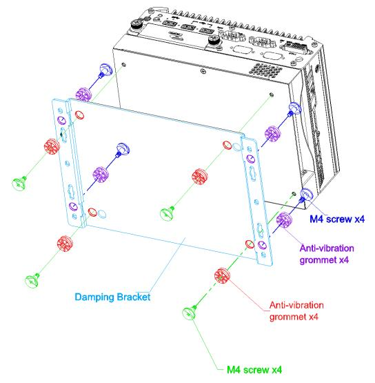
Referring to the illustration shown above, insert four anti-vibration grommets into locations on the side hinges indicated, secure the system using four M4 screws onto a flat surface in the vehicle.
