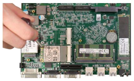
Insert on a 45° angle and secure using the screw provided
