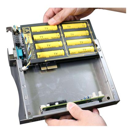
Remove the new supercapacitor UPS module out of the delivered enclosure/ static bag. Gently inserted it into the Cassette module. Make sure the PCIe gold fingers and panel are inserted properly.
