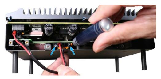
Release screws on the 3-pin connector
