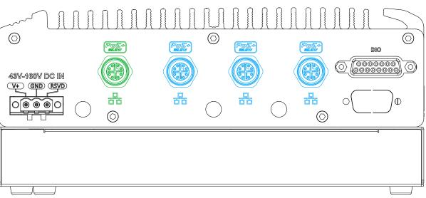
The system offers four PoE+ GbE ports via M12 X-coded connectors on the front panel. The ports are implemented using Intel<sup>®</sup> I210 controller and the port indicated in **green** supports Wake-on-LAN.
