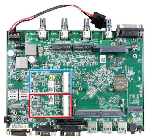
To install the mini PCIe module, insert the module on a 45° angle and secure the module using the screw provided.
