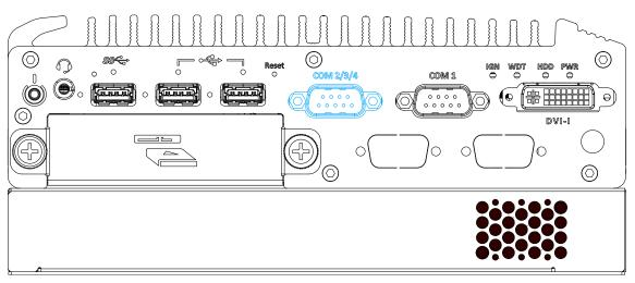
Implemented using industrial-grade ITE8786 Super IO chip (-40 to 85°C) and provide up to 921600 bps baud rate, the second D-Sub male connector (COM2/ 3/ 4) can be configured in BIOS as single RS-422/ 485 port (COM2) or three 3-wire RS-232 ports (COM2/COM3/COM4). Please refer to <u>COM2/ 3/ 4 Port Configuration</u> for configuring operation mode. An optional 1-to-3 Y-cable is available to connect three RS-232 devices.
