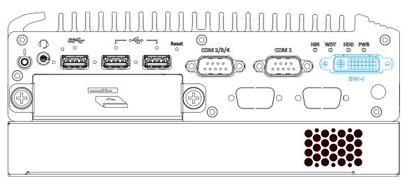
The system features a DVI-I connector on its front panel that is also compatible with VGA signals. The DVI and VGA outputs are directly driven by integrated Intel HD graphics engine and support up to 1920 x 1080 resolution.
