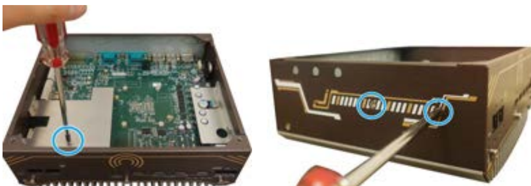
A screw on top of the heatsink
