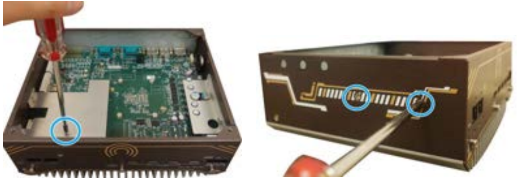
A screw on top of the heatsink
