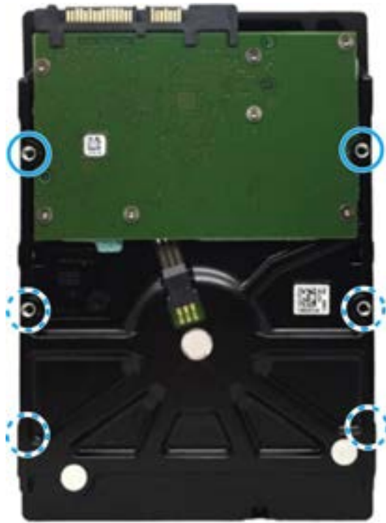
3.5" hard drive mounting holes
