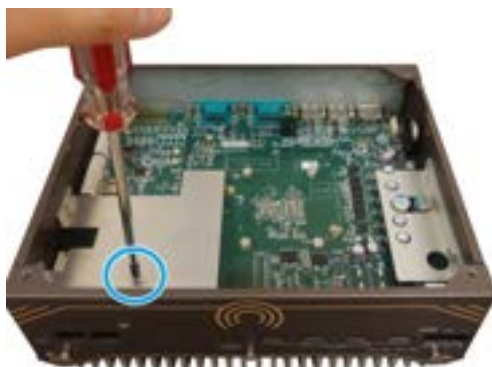
A screw on top of the heatsink
