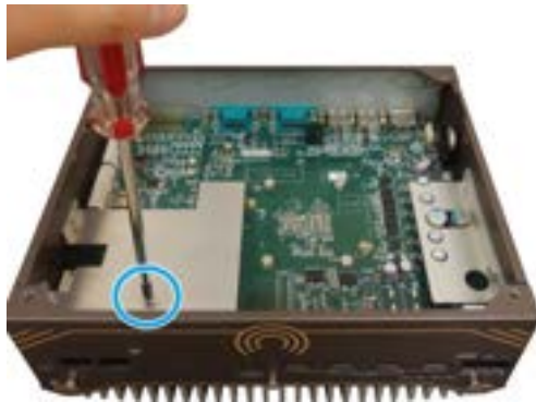
A screw on top of the heatsink
