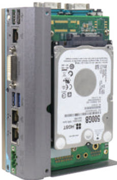
▲ POC-300 with MezIO® - R11 and 2.5" HDD
