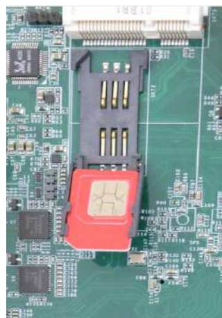
Insert SIM with pins facing upward
