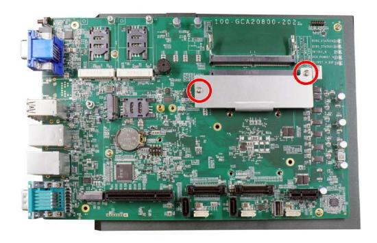
Screws on the memory module's heatsink
