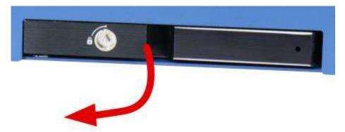
3. Insert the HDD/ SSD (with labels facing up) and the SATA connector end towards the slot, insert it 3/4 of way in and use the lever to fully push the HDD/ SSD into the slot. You should hear a click sound to ensure the HDD/ SSD is properly inserted and engaged.
