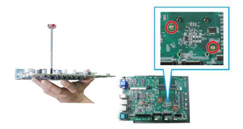
Hold CPU retention bracket firmly and turn the motherboard around
