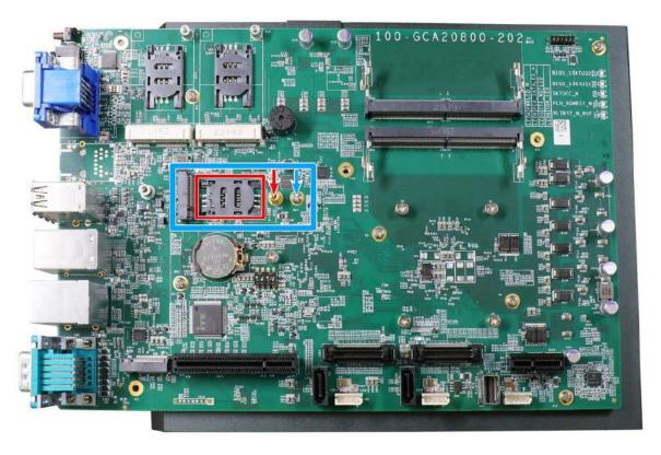
The system has an M.2 2242/ 3052 slot (indicated in **blue rectangle**) with a 5G/ 4G SIM slot (indicated in **red rectangle**). A copper standoff is provided for you to secure onto the motherboard into the **red arrow** location for an M.2 2242 module, or into the **blue arrow** location for an M.2 3052 module. By installing a 5G or 4G M.2 module and SIM card, you can access the internet via the provider's network.
