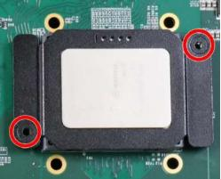
Screw holes for CPU retention bracket
