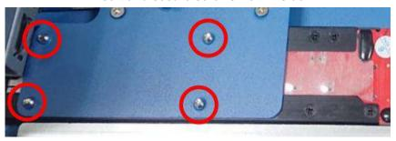
Screws secured inside-out
