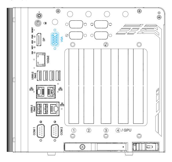
The VGA port is the most common video display connection. The VGA output supports up to 1920x1200@60Hz resolution.
