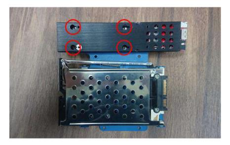
Insert and secure screws from inside
