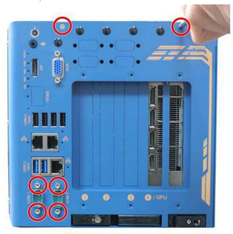
2. Remove six screws indicated on the side panel.
