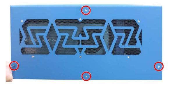
7. Secure the screws indicated on the top of the enclosure.
