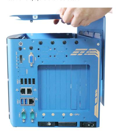
Place L-shape side panel onto the enclosure
