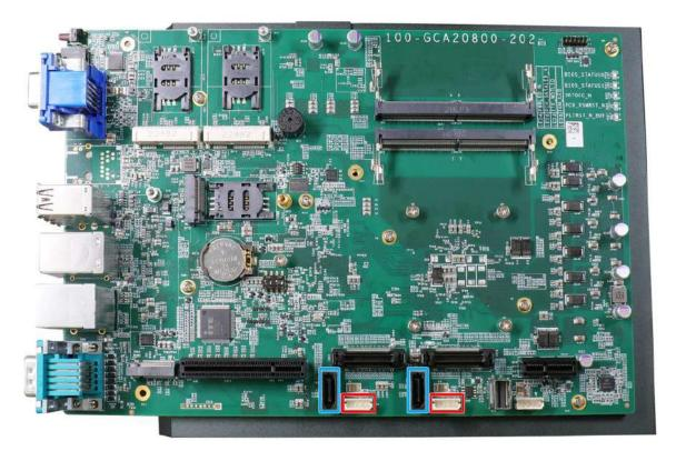
The system provides two SATA ports which support Gen3, 6 Gb/s SATA signals. Each SATA port (indicated in blue) features a 7-pin SATA connector and a 4-pin power connector.
