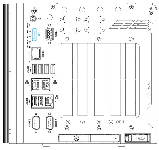
The DisplayPort (DP) output is a digital display interface that mainly connect video source and carry audio to a display device. When connecting a DP, it can deliver up to 4K UHD (4096 x 2304) in resolution. The system is designed to support passive DP adapter/ cable. You can connect to other display devices using DP-to-HDMI cable or DP-to-DVI cable.
