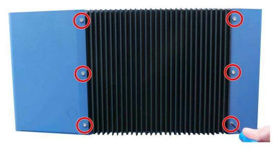
9. Gently lift and separate the heatsink and motherboard from the enclosure.
