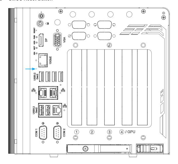
Positioned between 10GbE and USB ports, indicated by the **blue arrow**, the CMOS Reset button is used to manually reset the motherboard BIOS in case of system halt or malfunction. To avoid unexpected operation, it is purposely placed behind the panel. To reset, please use the tip of a pen, press and hold for at least 5 seconds to reset the BIOS.
