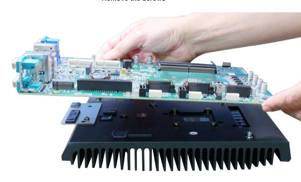
Separate the motherboard from the heatsink
