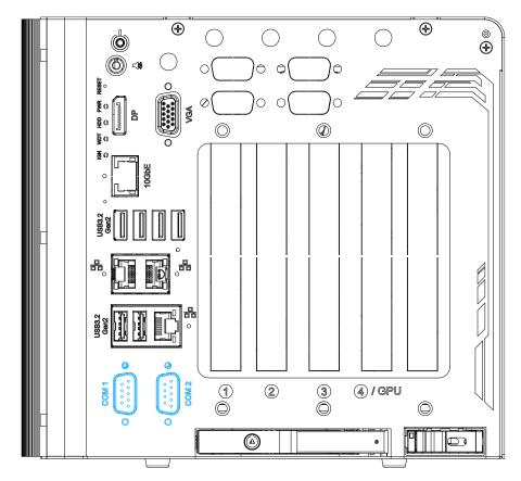
The two COM ports are implemented using industrial-grade ITE8786 Super IO chip (-40 to 85°C) and provide up to 115200 bps baud rate.
